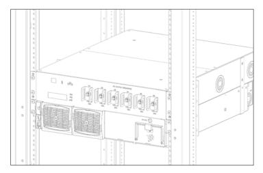
Fix the System in the cabinet with supplied mounting screws.
