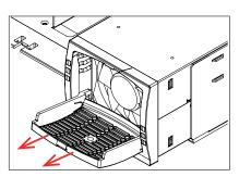
C) Use the cover as a handle to remove the module
