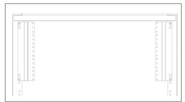
Fix the bracket with supplied mounting screws.
