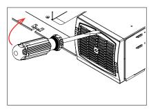
A) Use screwdriver to release the latch
